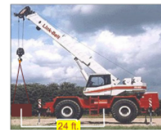
When actual radius is between listed values, use capacity for the next longer radius.
